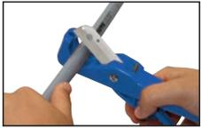
1. Cut the pipe square and straight with the Buteline pipe cutter.
