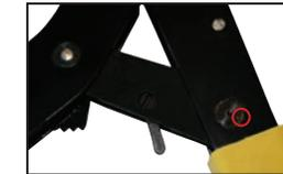
1. Identify the position of the adjuster cam by locating the dot on the hexagonal end of the cam.
