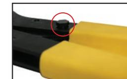
4. Push the adjuster cam out from the circlip side until the hexagonal head of the cam disengages from the handle, and turn the cam anticlockwise, so that it is moved around 1 flat of the hexagon.
