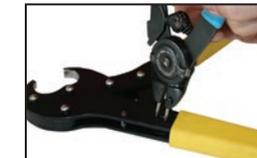
2. Turn the tool over and remove the circlip securing the adjuster cam.
