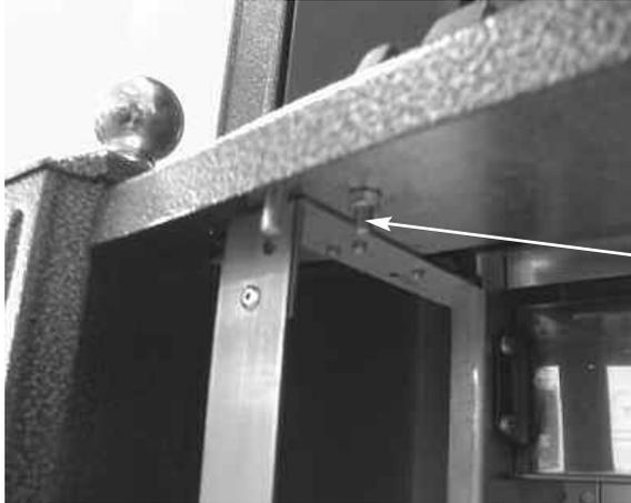
Front bezel retaining screws (1 off each side)
