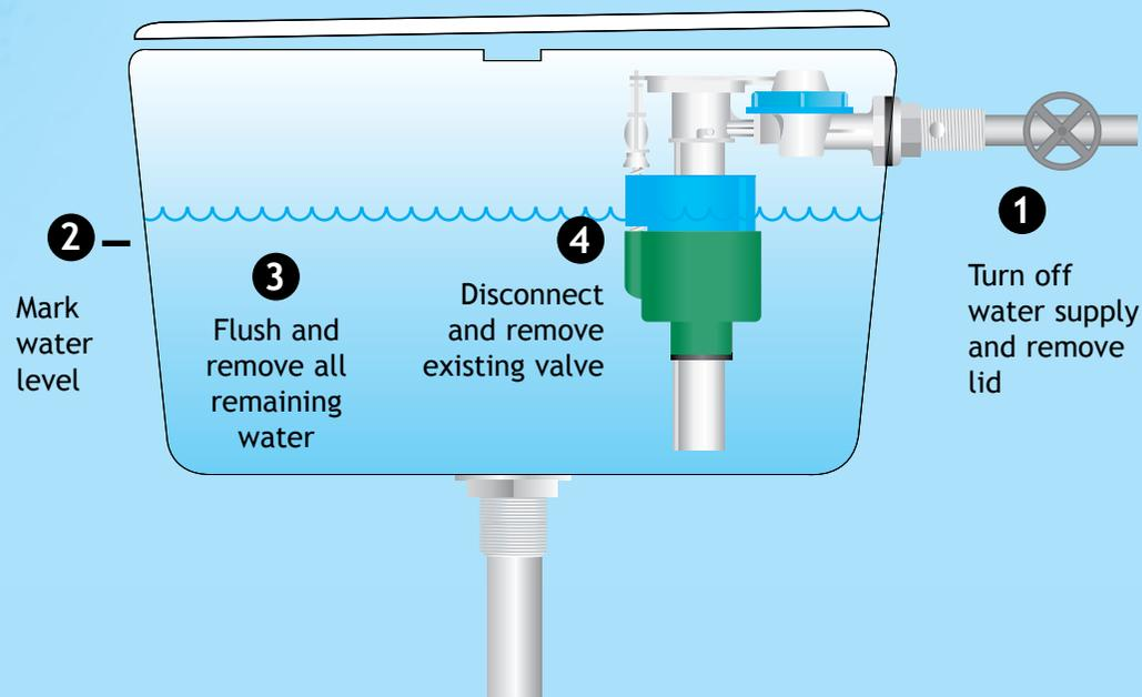
\*Valve can be fitted on either side of cistern.
